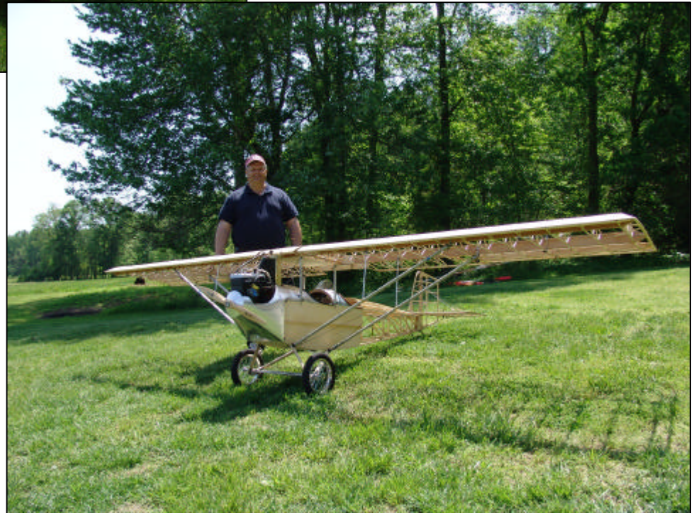
(above) Bill Setzler brought his 1/2-scale Pietenpol, in-the-bones, for display at the Fly-In. Bill began this impressive scratch-build project over a year ago. When completed, the 14' model will be powered by a Sachs 5.8 (hidden under the scale replica engine), and weigh in the neighborhood of 75 lbs.
